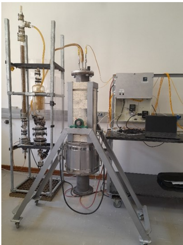
Photo: Modified Bubbling Bed Gasifier and Condenser
